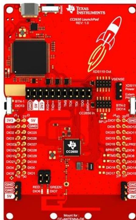
The device uses an ARM Cortex M3 main processor and up to 48-MHZ clock speed. For more information about the CC2650:
