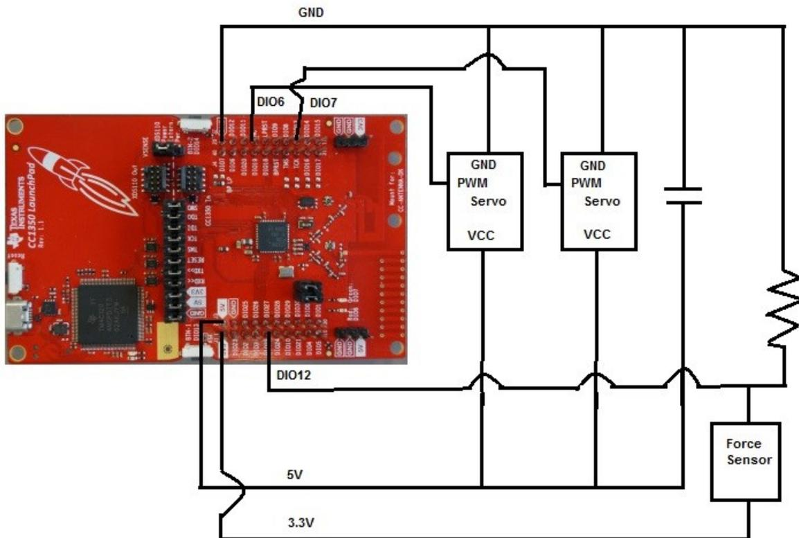
Figure 1: Circuit description - For clarity DIO pins are spread out, and do not match their actual locations on the board.
