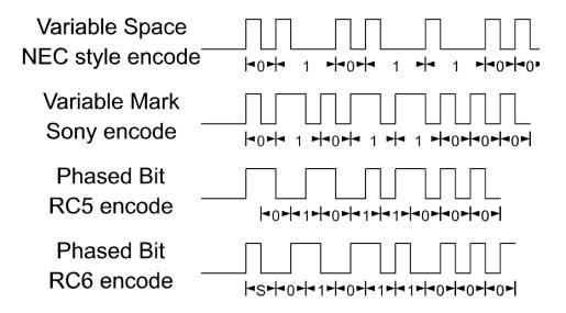
In this illustration the top part illustrates the variable space encoding used by NEC and most other protocols. The second row shows the Sony system which uses variable marks instead of variable spaces. It is relatively easy to look at a graph of those signals and see that they are either variable spaces or variable marks. Once you get good at it, you can look at timing values and figure out the bit patterns in your head.
