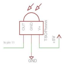
Note that all of our examples presume +5 volt supplies however some Arduino systems run at 3.3 volts. These schematics should also work at 3.3 volts. It is critical that you do not use a 5 volt supply on your receiver if you are connecting to a 3.3 volt system.
