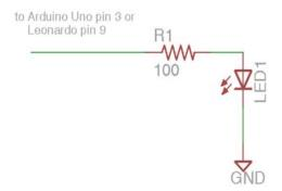
Make sure you get the polarity of the LED correct. The shorter of the two leads should connect to ground. The longer lead connects to the resistor which in turn connects to the Arduino.
