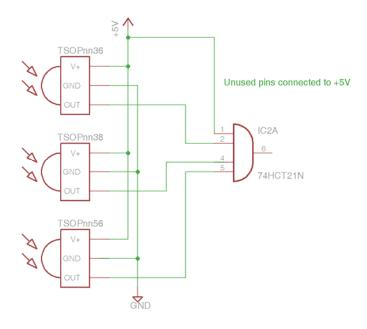
You would connect the output pins of each receiver to a logical AND gate. Here we are using a 74HCT21N quad input AND gate. You could use a 74HCT08N dual input that come 4 to a package. The 74HCTxx series is a CMOS chip that will operate at 5V TTL compatible levels suitable for use with Arduino at 5V. If you have any unused input pins on the gate you should tie them to +5.
