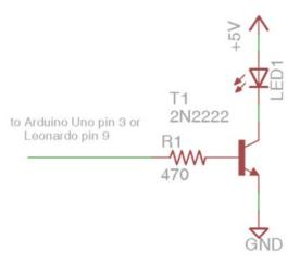
Because Arduino pins cannot produce much current we recommend you use an NPN transistor as a driver circuit if at all possible. On the left is a schematic of what that looks like.
