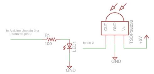
Be sure to get the polarity correct on the LED. The shorter of the two leads connects to ground and the longer one connects to the resistor.
