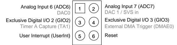
Figure 21: Functionality of the 6-pin expansion connector (U28).
