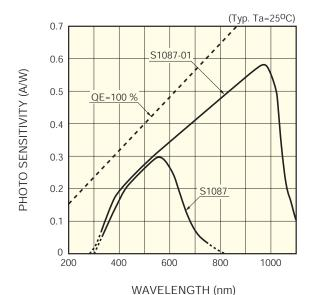
Figure 19: Photo Sensitivity of the Light sensors on Tmote Sky (from Hamamatsu)
