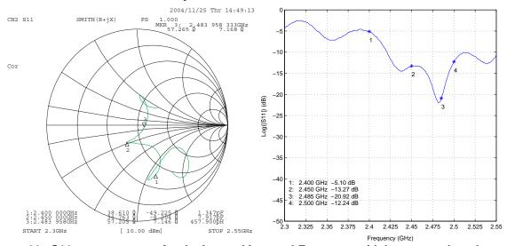
Figure 11: S11 measurements for the internal inverted-F antenna with battery pack underneath
