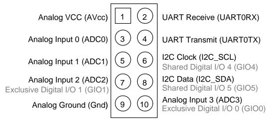
Figure 20 : Functionality of the 10-pin expansion connector (U2).
