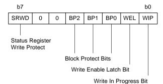
Figure 15: ST M25P80 Status Register contents (from ST).
