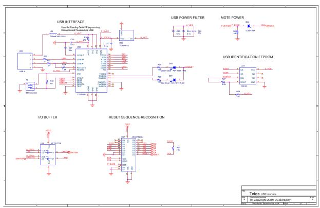
Figure 4: Schematics for the Tmote Sky module
