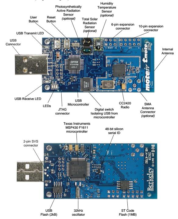
Figure 1: Front and Back of the Tmote Sky module
