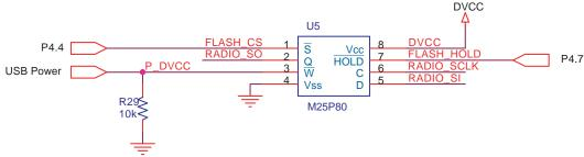
Figure 14: External serial flash schematic
