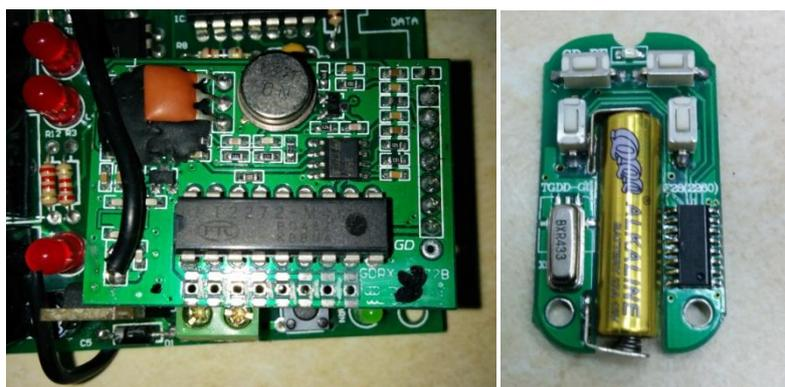
Figure 4: Detailed View on the receivers' decoder and remote controls' encoder
