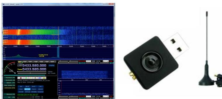
Figure 5: Left - HSDR main window , Right - the RTLSDR we used
