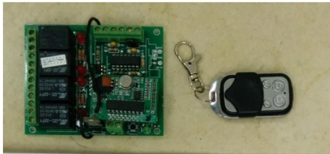
Figure 3: The receiver/transmitter Kit we used
