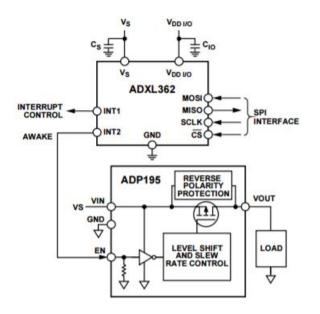
In order to transfer this data the sensor and the MCU are connected in a certain way that follows the SPI protocol. We connected the sensors MISO to the board according to the formal datasheet, as well as MOSI, CS (chip select), clock and the appropriate voltages.
