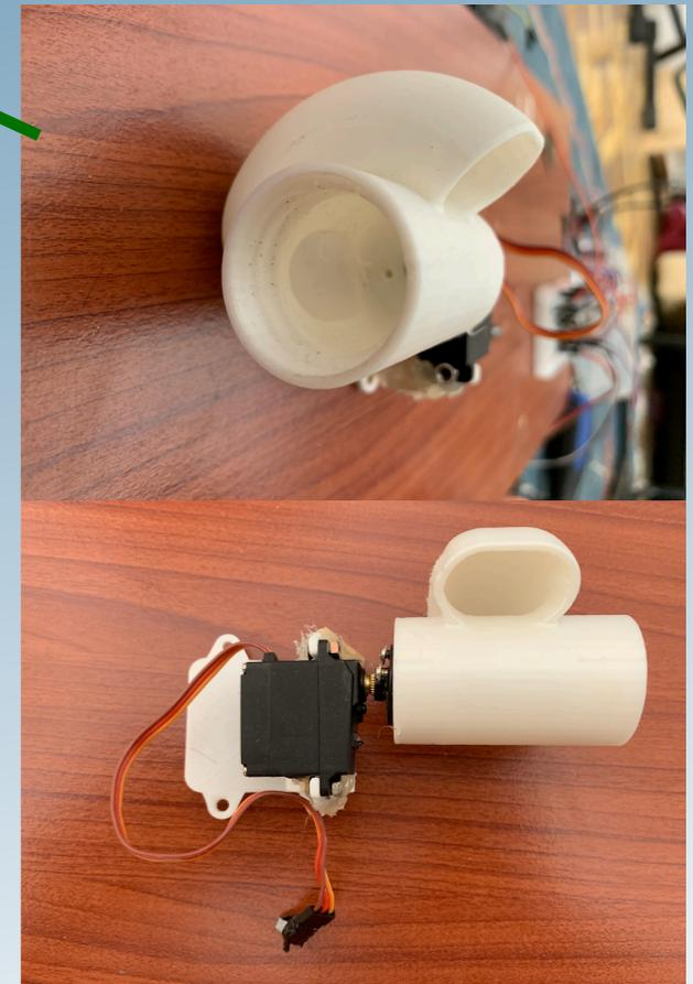
3D Printed cap attached to Servo Motor
